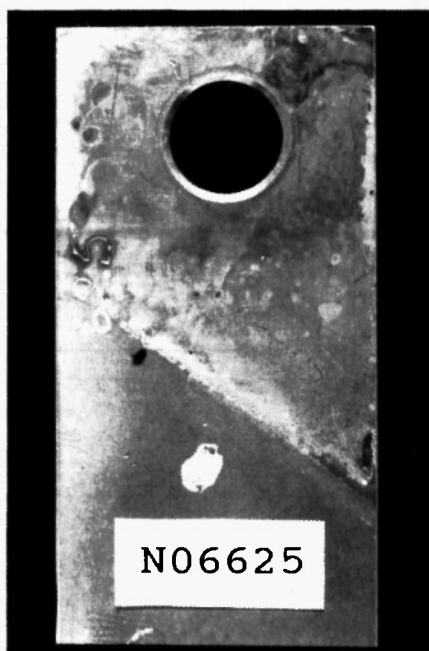
Fig. 11: Vapor phase corrosion on N06625 nickel base alloy
