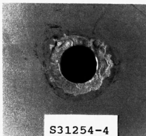
Fig. 8: Crevice corrosion on S31254 superaustenitic 6 Mo steel
