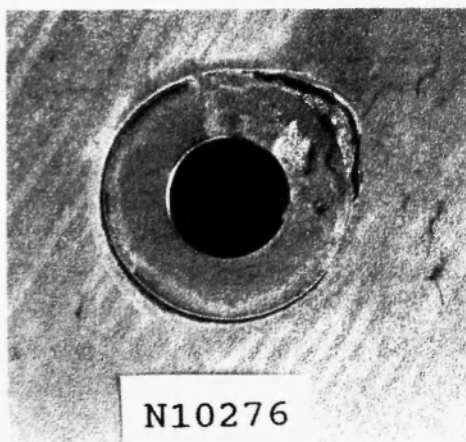
Fig. 10: Crevice corrosion on N10276 nickel base alloy
