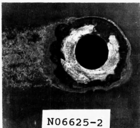
Fig. 9: Crevice corrosion on N06625 nickel base alloy
