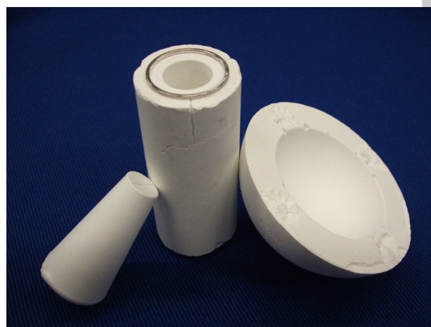
Figure 1: Different geometries of bone graft substitutes; an incorporated reinforcing metallic structure can be seen within the tube bone graft substitute (see center)
