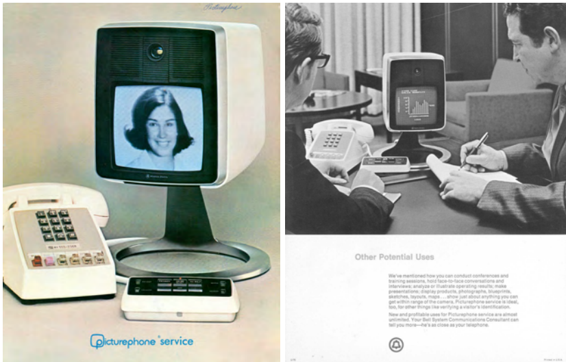
Figure 5 a–b: Images of the AT&T Picturephone Mod-II with accessory pieces, 1970 (left); and as a display device for computer output, 1970 (right)
