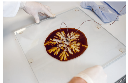
Hele-Shaw experiment Department Petroleum Engineering (DPE) laboratory University of Leoben, 2020
