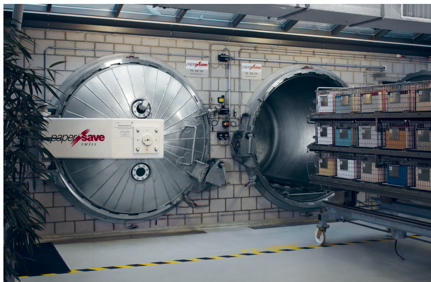
Fig. 1: The papersave swiss facility in Wimmis on the premises of the Nitrochemie Wimmis AG, in operation from 2000 to 2022. Interior of the papersave swiss facility. The treatment chambers. Photo: Nitrochemie Wimmis AG
