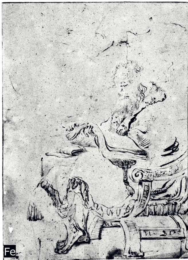
Fig. 7: Reading Old Man . The element distribution of iron (Fe) determined with an X-ray fluorescence scanner indicates a signature with an iron-containing material, iron gall ink. Image: Klassik Stiftung Weimar, Graphische Sammlungen, graphics: Uwe Golle
