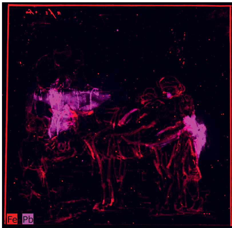
Fig. 9: The Levite and the Dead Concubine , elemental distributions of iron (Fe) and lead (Pb). Image: Klassik Stiftung Weimar, Graphische Sammlungen, graphics: Carsten Wintermann
