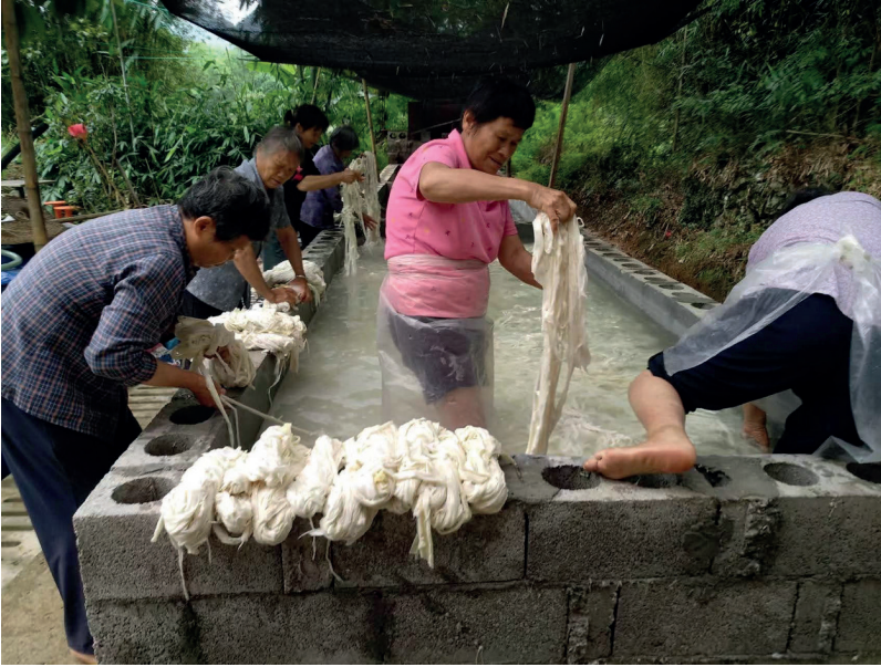
Fig. 7: Rinsing the yarn that has been boiled
