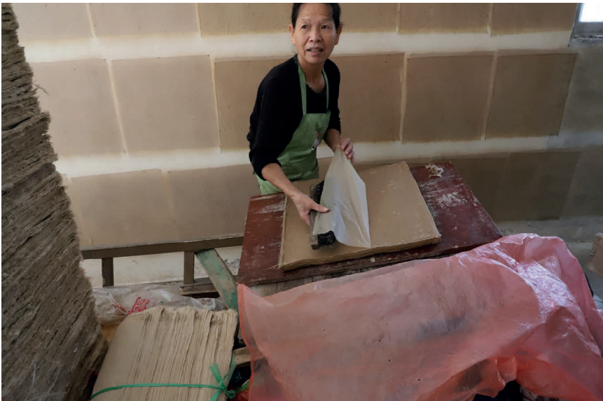
Fig. 14: Peeling off the half-dried paper sheets
