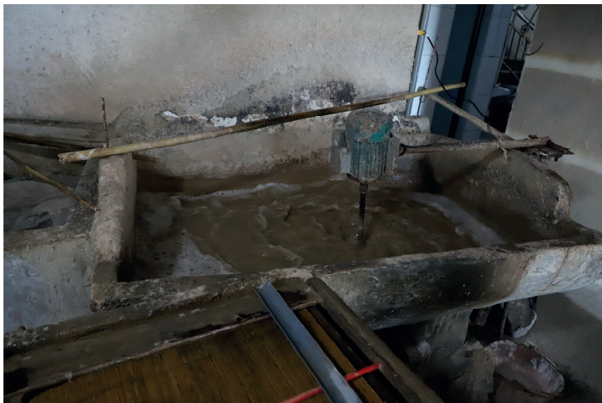
Fig. 9: Fibre pulp being stirred in the trough
