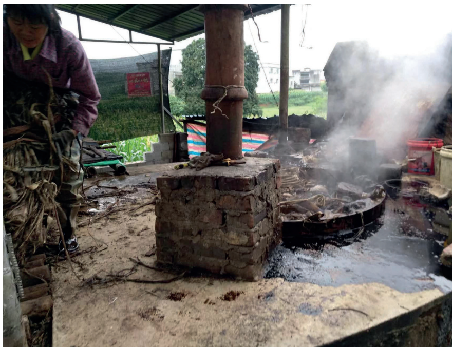
Fig. 6: Boiling the raw yarn
