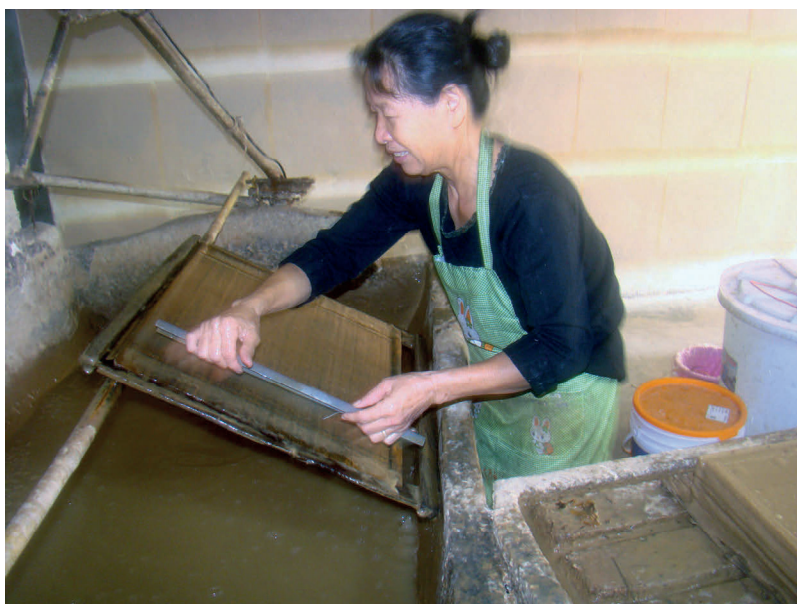
Fig. 12: Trimming the edges of the wet paper
