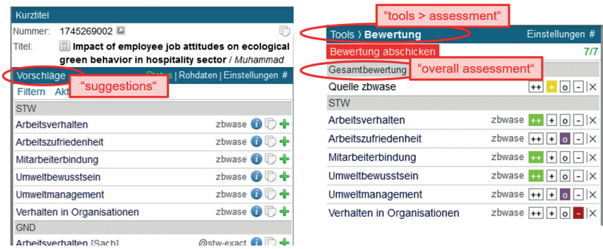
Figure 14.4: Partial screenshot of DA-3 where users can see and assess machine-generated suggestions during their subject indexing work
