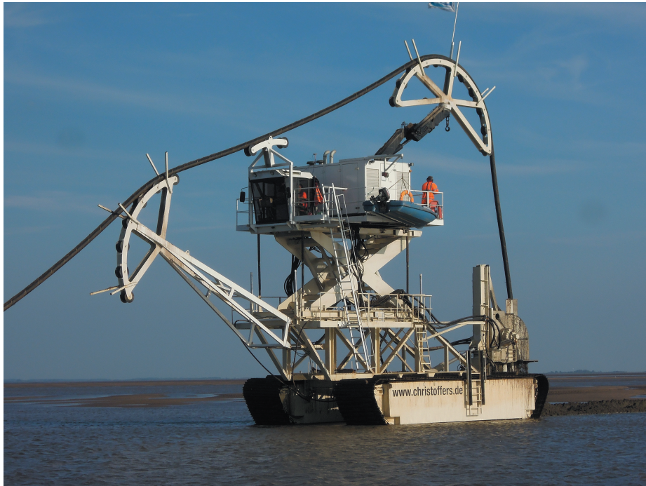
Fig. 1.1: This modern submarine cable trencher, a special machine for laying undersea cables offshore, weighs more than 100 tonnes.
