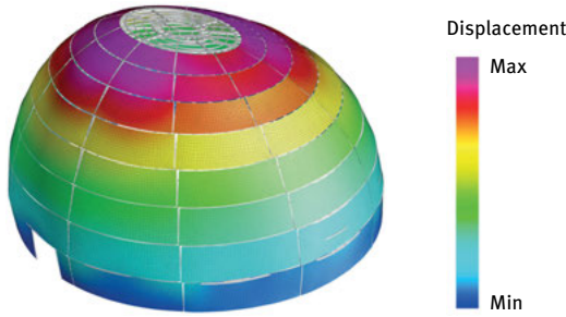
Fig. 13: Horizontal layout: Natural frequency analysis, first mode 2.1 Hz.
