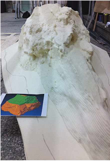
16 | CNC milling process of rocks for Alice Channer's Burial , 2016.
