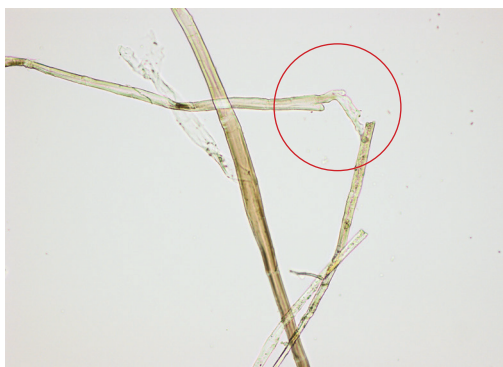
Fig. 7: Daphne/Wikstroemia fibres with the irregular shape of the fibre ends.
