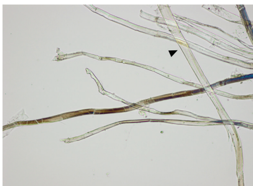
Fig. 8: Stelleria fibres with ribbon-like shape (arrowheads) from Naxi manuscript 101502.
