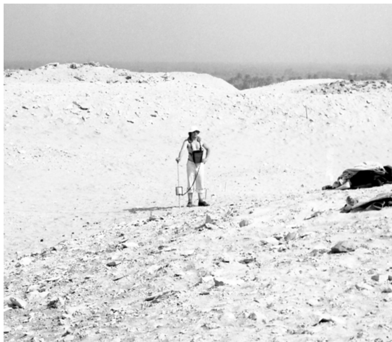
Fig. 3: Abusir. Vladimír Hašek taking measurements with a proton magnetometer.
