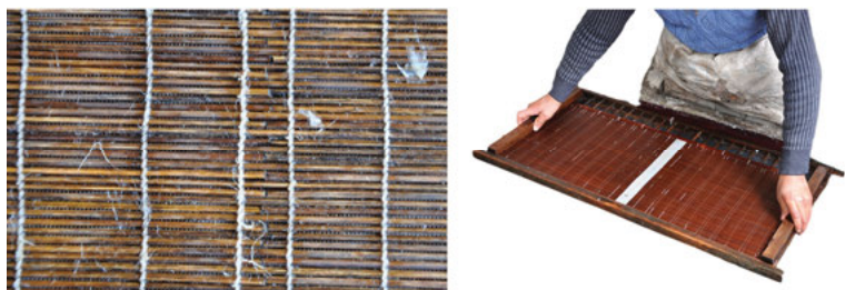
Fig. 5c: Laid paper made with the mould equipped with the bamboo sieve. Figs 5a–c: Photographs by Agnieszka Helman-Ważny, diagrams by Dorota Helman.
