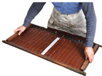
Fig. 5c: Laid paper made with the mould equipped with the bamboo sieve. Figs 5a–c: Photographs by Agnieszka Helman-Ważny, diagrams by Dorota Helman.
