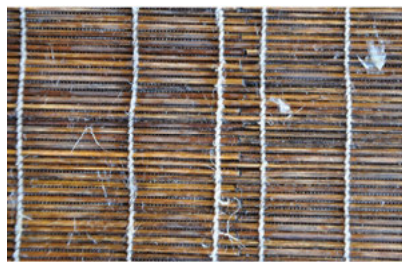
Fig. 5c: Laid paper made with the mould equipped with the bamboo sieve. Figs 5a–c: Photographs by Agnieszka Helman-Ważny, diagrams by Dorota Helman.
