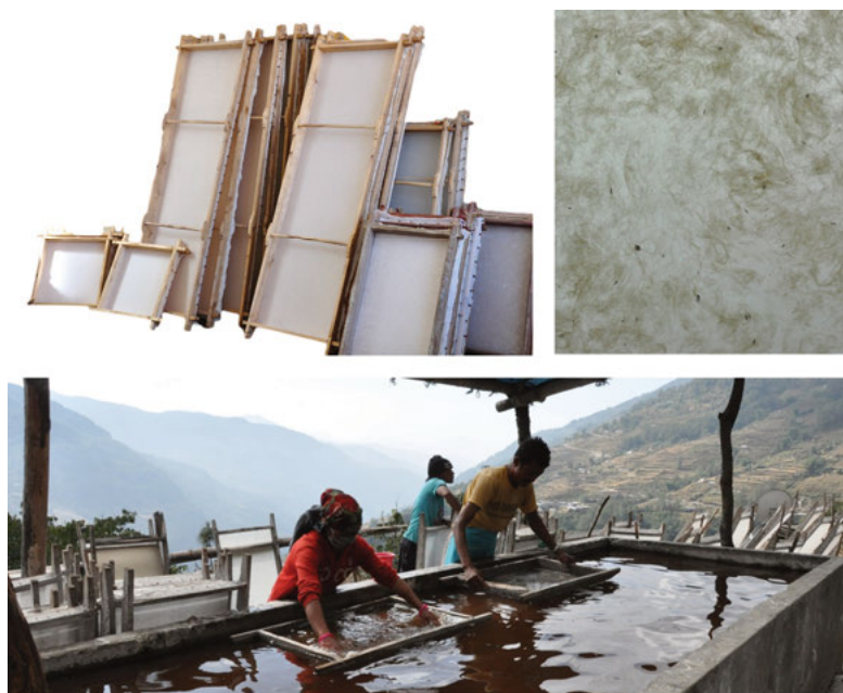
Fig. 4b: Technology of papermaking with a textile sieve.
