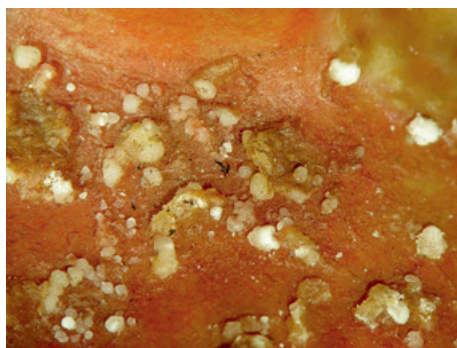
Fig. 5: Microscopic photography of wax surface with efflorescence and crystalline coating induced by climatic fluctuations, 1955. Moulage from the collection of Deutsches Hygiene Museum Dresden.
