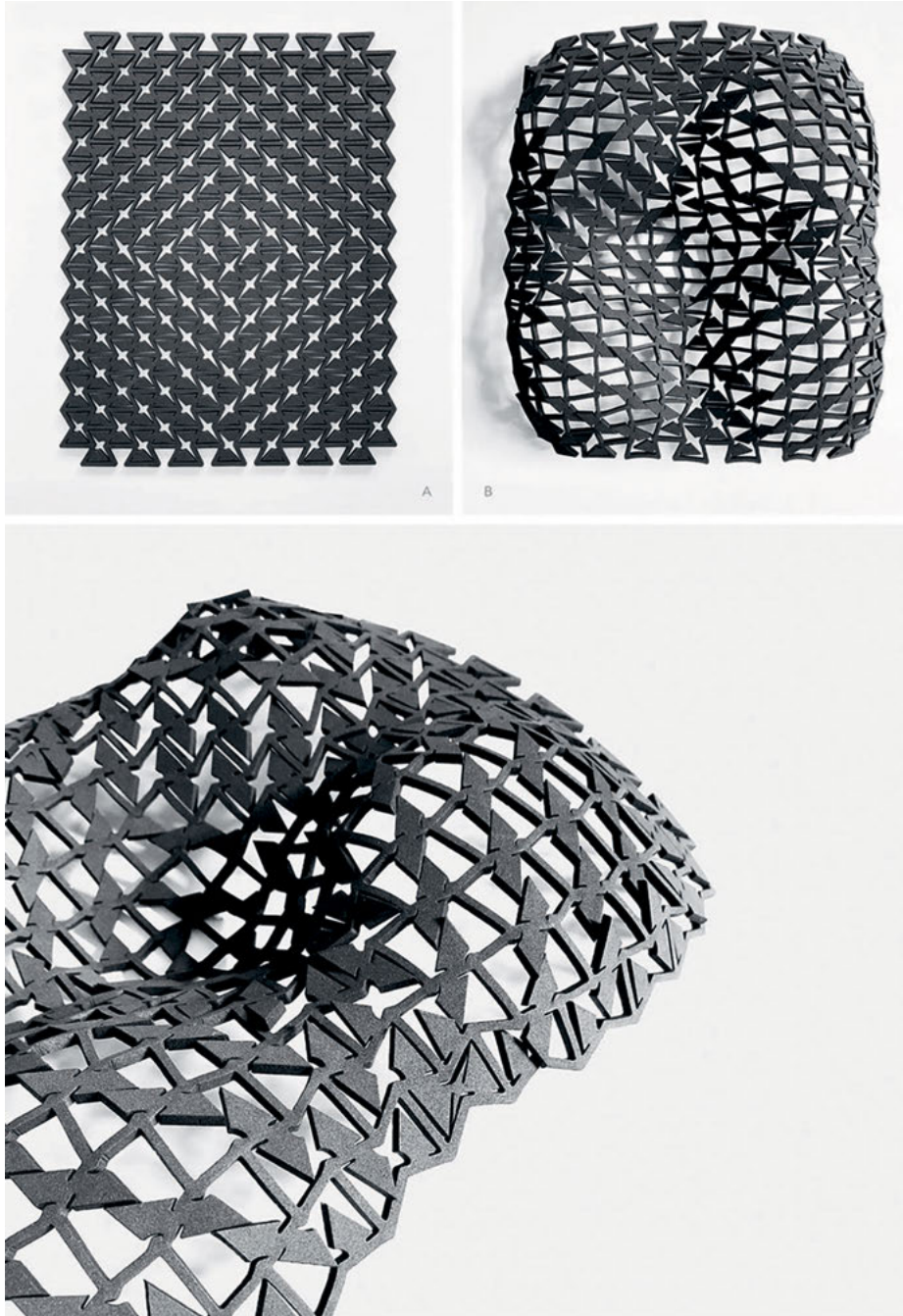
Fig. 6: An auxetic sheet composed of mirrored cells grouped into four distinct quadrants morphing into a quadruple dome.
