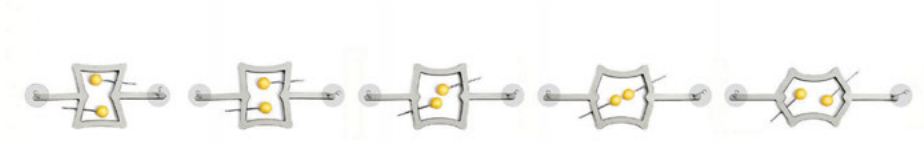
Fig. 3: An inverted hexagonal cell, at increasing stretching, externally fixed to a support (gray circles). The yellow pins showcase the rotation of two opposite inclined walls upon stretching.
