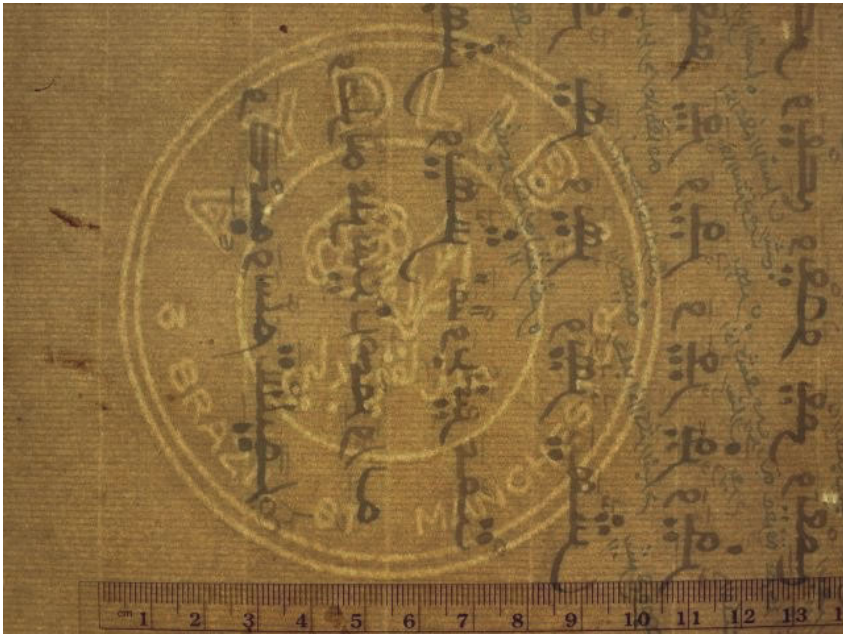
Fig. 10: The YDLIBI watermark/countermark combination made by a dandy roll on machine-made paper. (Falke 14).
