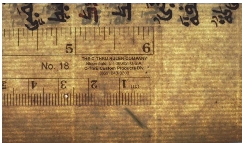
Fig. 7: A cloudy sheet, uneven in its formation, with a grass stem inclusion. (Private collection).
