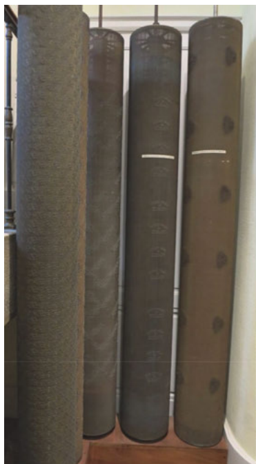
Fig. 9: Dandy rolls (with detail) produce watermarks and countermarks and can easily be changed on both cylinder and continuous machines. These machines can also produce large quantities of paper from the same dandy roll and the same roll can be used for decades. (Musée Canson-Montgolfier, Annonay, France, 2013).
