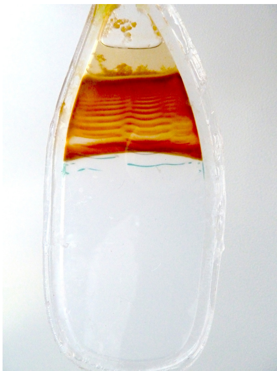
Figure 8.15: Liesegang ring plates were constructed from two perspex plates separated by a 0.5 cm gap sealed with silicone. Alkalinised agarose at 2% v/v was introduced into an apical gap in the plate system and allowed to cool for an hour. A solution of iron II, iron III and copper II salts was introduced into the apical reservoir. Within a few hours, precipitates could be seen moving through the plates, and produced striking banding patterns that continued to evolve over the duration of the three-month installation. Photograph, Rachel Armstrong, July 2010.
