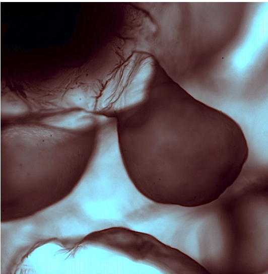
Figure 8.39: Osmotic forces rupture the Traube cell membranes that form around the copper II sulphate crystal and immediately heal as the salt solutions come into contact with each other. Micrograph, magnification 40×, Rachel Armstrong, February 2009.
