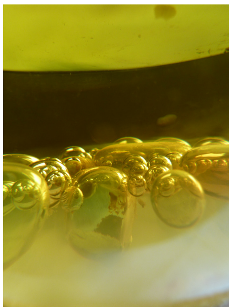
Figure 8.6: Modified Bütschli droplets self-assemble at the interface between green olive oil (above) and yellow-tinted DEPP (below) and are clearly visible in a gallery setting. Photograph, Rachel Armstrong, April 2011.
