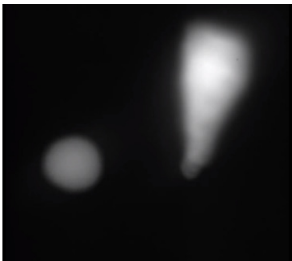
Figure 6.8: An osmotic cast is observed under fluoroscopy from the droplet in Fig. 6.7, which has been pre-stained using a fluorescent dye (fluorescein 0.01 M at pH 9). The structures are observed under a red light filter to pick up the green light emitted by the stain. The images show that the residual osmotic structures appear to be soap crystal skins that encase an aqueous inner core. Micrograph, magnification 40×, Rachel Armstrong, February 2009.
