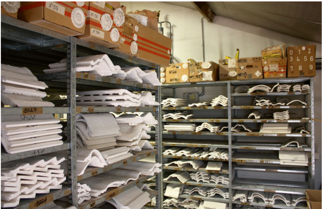
Plates Intro.15a–c The modern production process of plaster casts of/for decorative elements and of/for architectural surfaces (above left), surviving casts from Angkor Wat (above right, compare Pl.Intro.10b and 16a) and the storage of lightweight decorative elements (French: staff ) (below), photos taken at Maison Auberlet , successor of the original Auberlet & Laurent , which executed the decoration of the 1:1-scale version of Angkor Wat at the International Colonial Exhibition in Paris 1931 (Source: © Michael Falser 2010)
