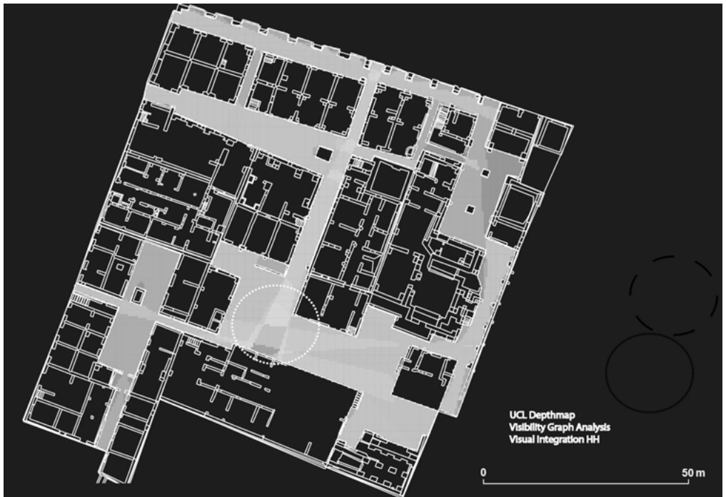
Figure 8 | VGA identifies the southern courtyard as the visually most integrated space (marked by a circle).
