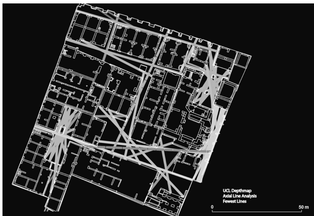
Figure 7 | The Insula's potential route matrix based on the longest and fewest lines; represented in greyscales. The movement spaces of the Terme del Faro are included in the analysis (Depthmap 7.12.00d; The Bartlett, University College London).
