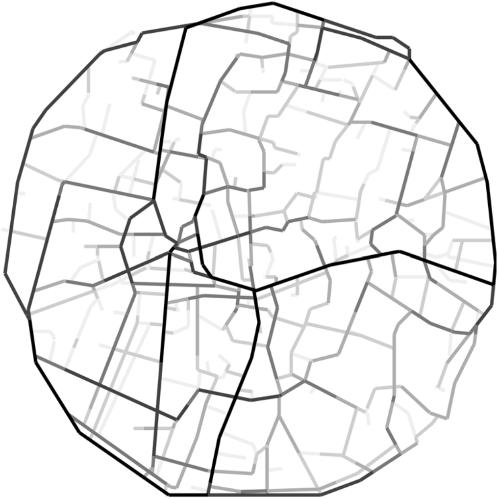
Figure 18 | Segment map show integration at unrestricted radius with the least angle change definition of distance for Nicosia within the walls (dark: strong/light: weak). In spite of the strong spatial difference in the background network, the system is structured by a deformed wheel core.
