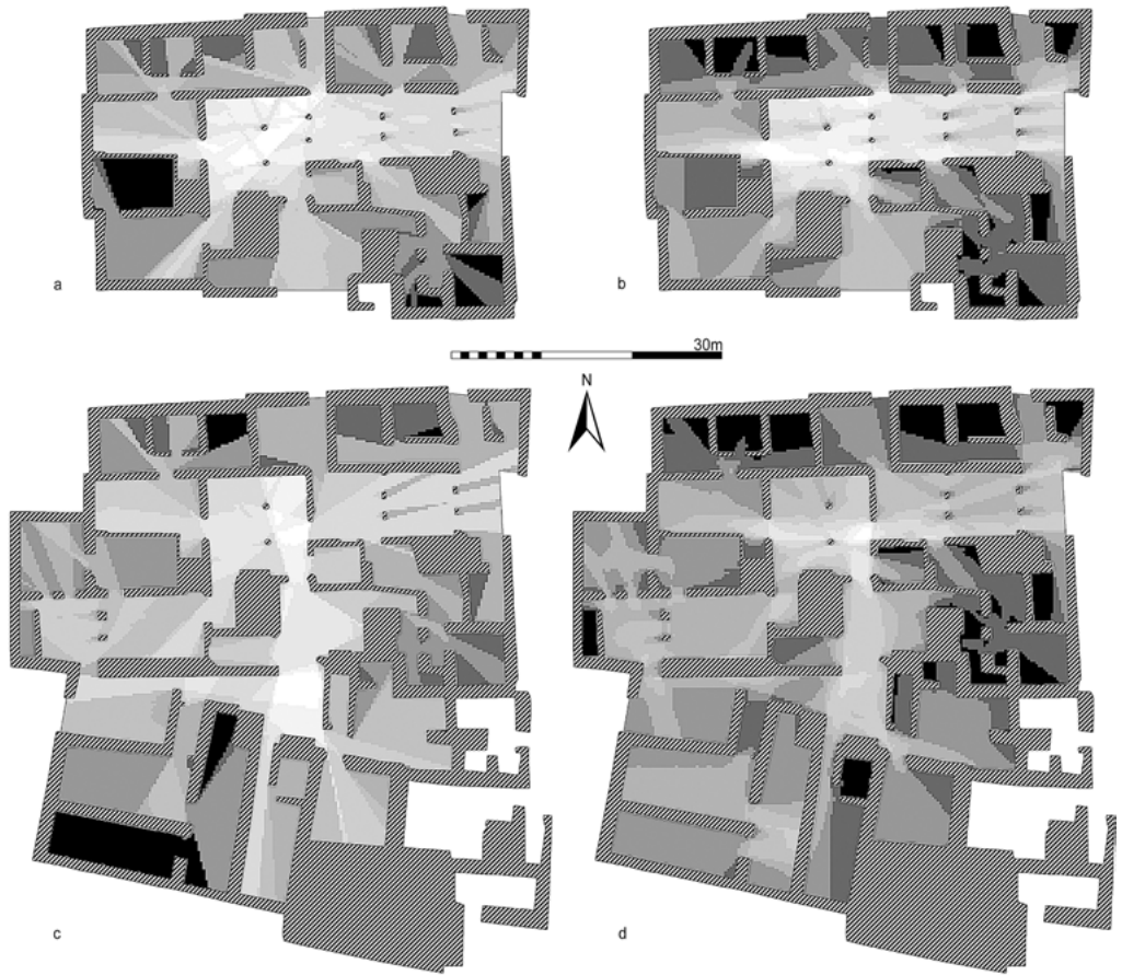
Figure 6 | Malia, Quartier Mu, Building A: a) plan of phase 1 with visual integration indicated by shading (lighter shading denotes higher integration); b) plan of phase 1 with visual connectivity indicated by shading (lighter shading denotes higher connectivity); c) plan of phase 2 with visual integration indicated by shading (lighter shading denotes higher integration); d) plan of phase 2 with visual connectivity indicated by shading (lighter shading denotes higher connectivity).
