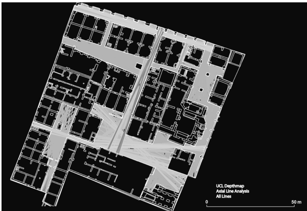
Figure 6 | Insula IVii: internal courtyards, including the movement spaces of the Terme del Faro; axial analysis (all lines) identifies the central passage leading from the portico to the southern courtyard as the visually most integrated space (graphs and analyses produced with Depthmap 7.12.00d; The Bartlett, University College London).
