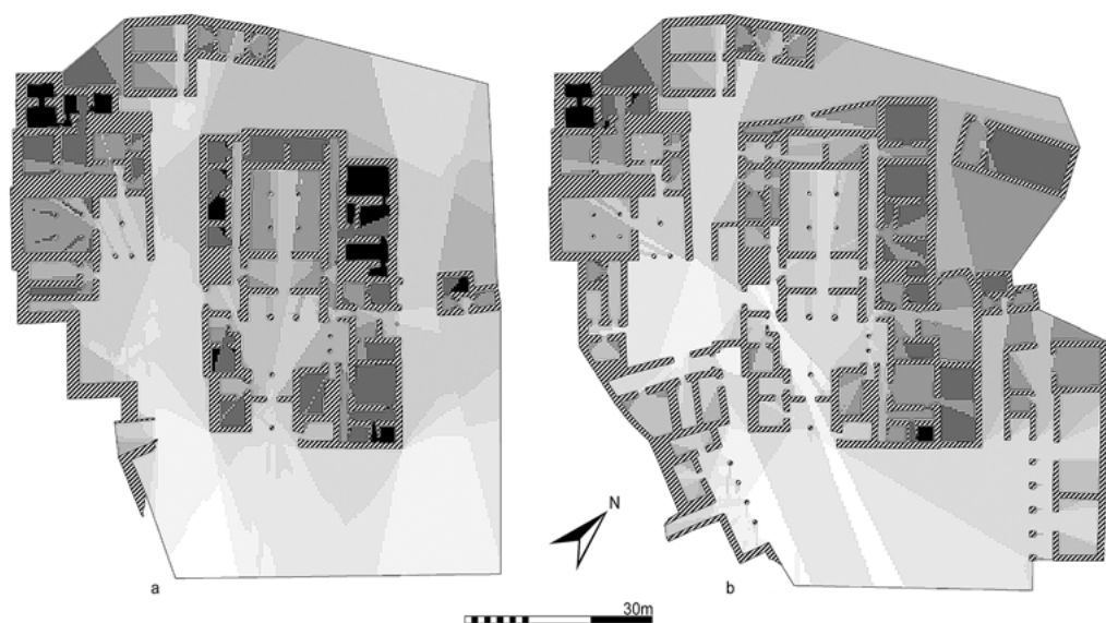
Figure 13 | Pylos, palace: a) plan of earlier building state with visual integration indicated by shading (lighter shading denotes higher integration); b) plan of later building state with visual integration indicated by shading (lighter shading denotes higher integration).
