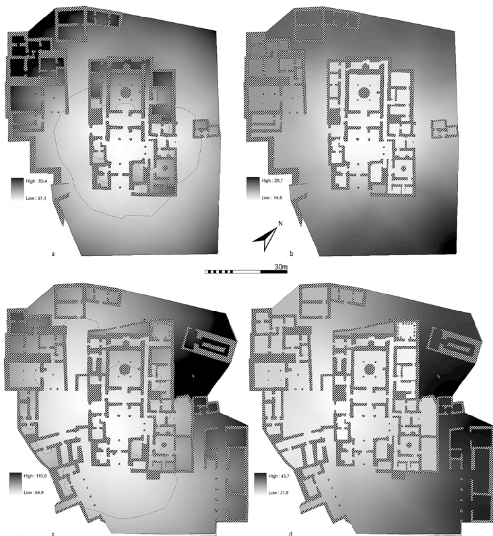
Figure 17 | Pylos, palace: a) AMD map of the earlier building state; b) STMD map of the earlier building state; c) AMD map of the later building state; d) STMD map of the later building state. The border of the metric integration core for each case is shown by a solid line.
