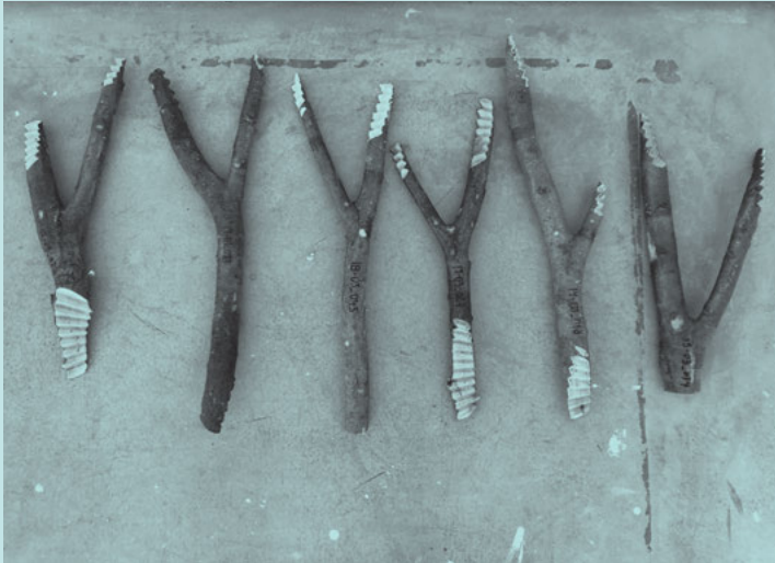
▲ CNC-processed hornbeam and beechwood branch parts prior to assembly, at the Angewandte Innovation Laboratory (AIL), 2019.
