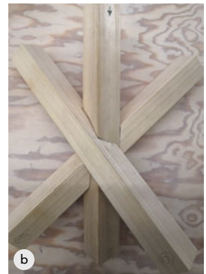
▼ Figs. 2a+b | Abb. 2a+b: Sample of a structural knot with three parts connected via half lap joints. The varying orientations of parts affect modifications of the standard form at the joint. a) Disassembled. b) Assembled.
