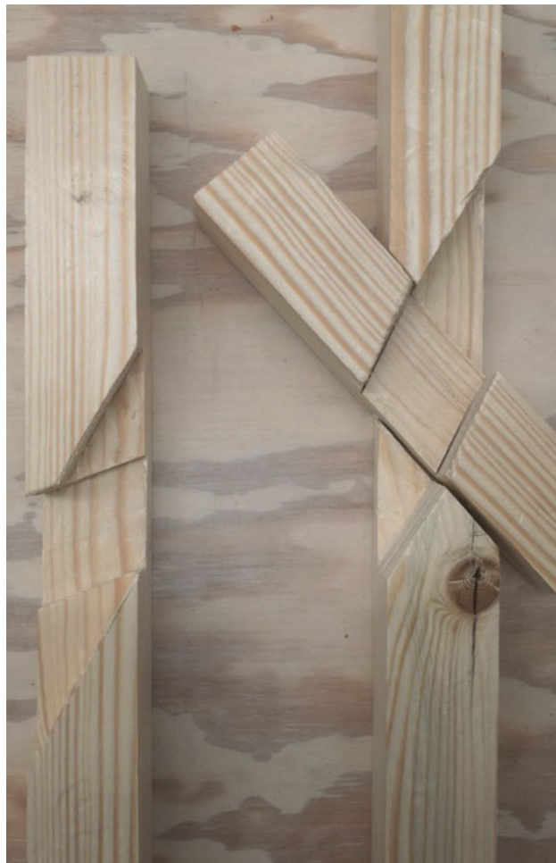
► Fig. 3b | Abb. 3b: Analog joint studies with spruce elements with a cross section of 5 \times 5 cm.
