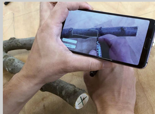
◀▲ Fig. 23 | Abb. 23: The smartphone app, developed by Ben James, makes it possible to 'map' digitally generated cutting lines onto physical branches. These lines are manually traced with a pen.
