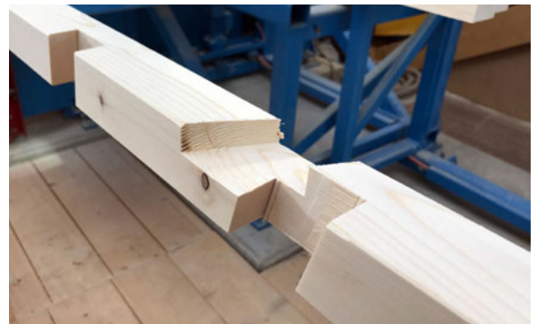
▼ Fig. 3b | Abb. 3b: Example of a joint for connecting three members. Image from the CNC production for the IS-2 installation at AIL, 2019.
