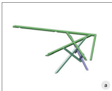
▲▲▲ Figs. 6a–c | Abb. 6a–c: A configuration of beams (a) is duplicated and rotated 180° (b) to form a complete structure (c).
