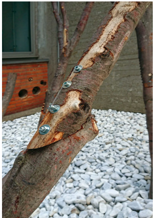
▲ Fig. 8 | Abb. 8: Comparison of a screwed and a bolted connection.
