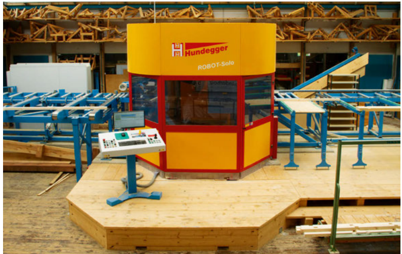
► Fig. 7 | Abb. 7: Hundegger Robot-Solo CNC truss-cutting machine at the Vocational School Murau, Austria, 2019.
