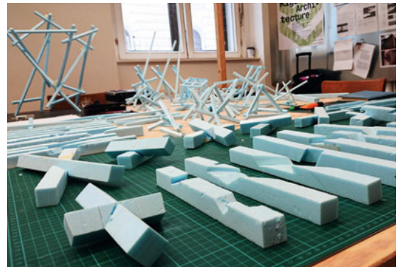
▲ Fig. 2a | Abb. 2a: Connection detail development with extruded polystyrene hard foam as a model making material.
