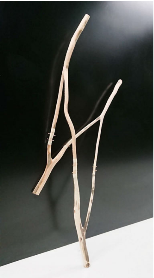
▲ Fig. 6c | Abb. 6c: Realization of one tetrahedral cell, built from four Y-shaped hornbeam and beechwood branch forks.
