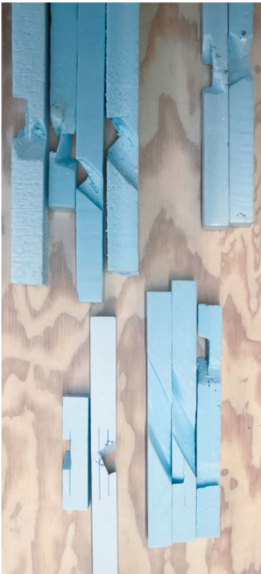
◀ Fig. 3a | Abb. 3a: Details of model elements from hard foam that were used to develop a joining system over the course of the student workshop with Jun Sato at the Angewandte 2018.
