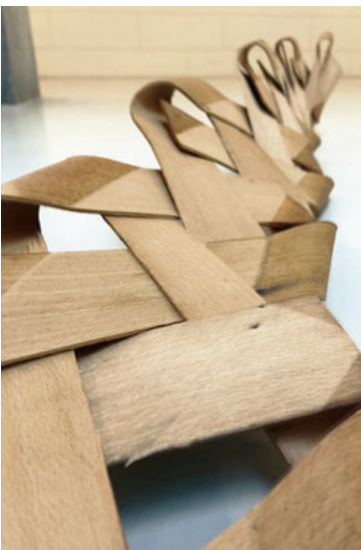
▼▼ Fig. 4b | Abb. 4b: Working models of grid-shell structures, made of interwoven surface strips.
