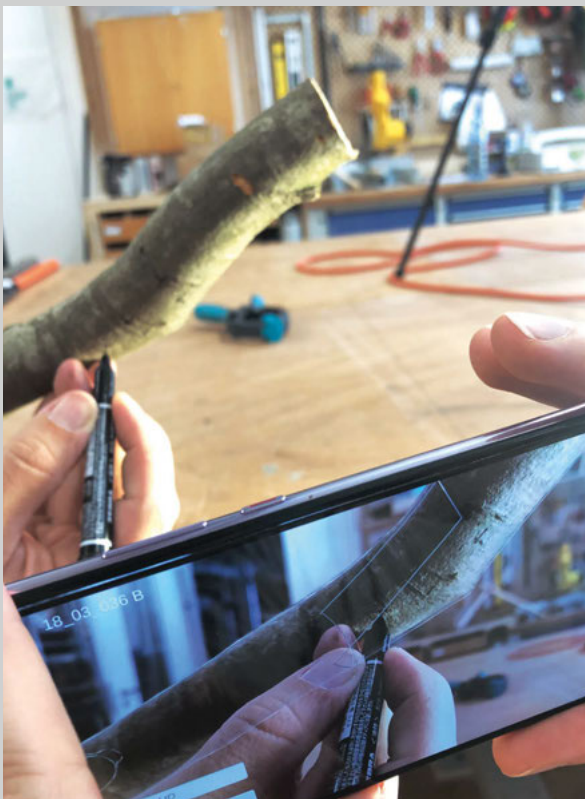
◀▲ Fig. 23 | Abb. 23: The smartphone app, developed by Ben James, makes it possible to 'map' digitally generated cutting lines onto physical branches. These lines are manually traced with a pen.
