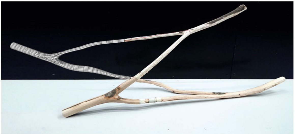
▲ Fig. 26a | Abb. 26a: Digital and physical models of four Y-shaped branches assembled into one tetrahedral module.
