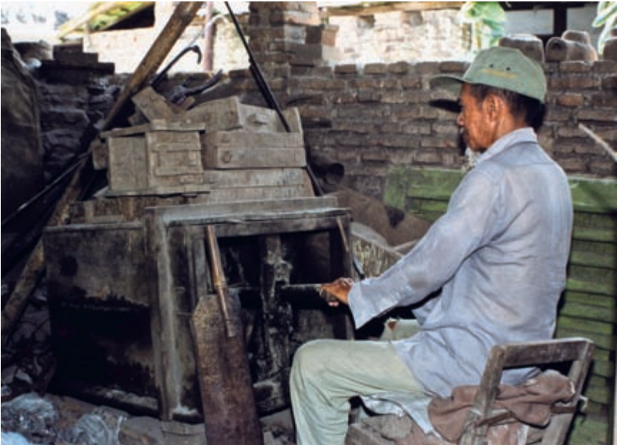
(opposite) Making a repoussé silver bowl in Kamasan village, Bali; the tool used by the smith is tipped with bell metal, a type of bronze.
