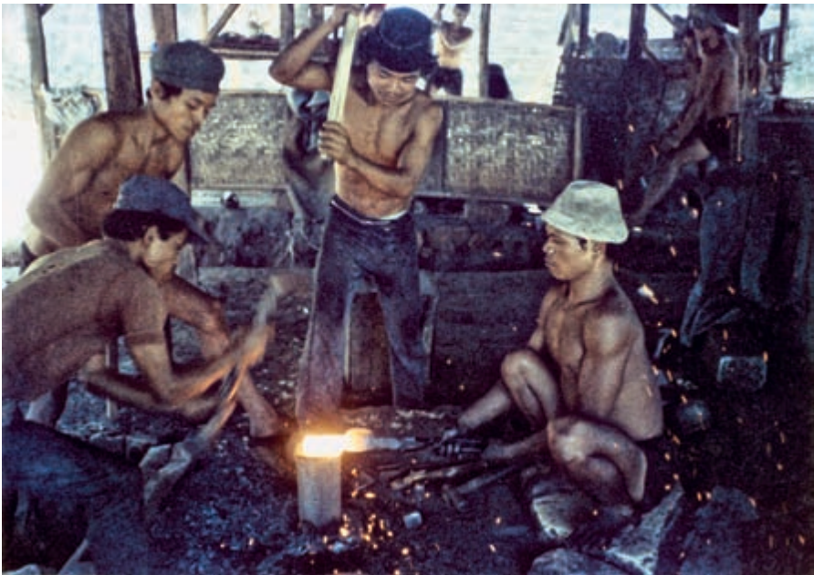
(opposite) An empu making pick-axes, Kamasan village, Bali; note that there are two quenching troughs in the foreground, a bamboo trough filled with used motor oil and a stone trough filled with water.
