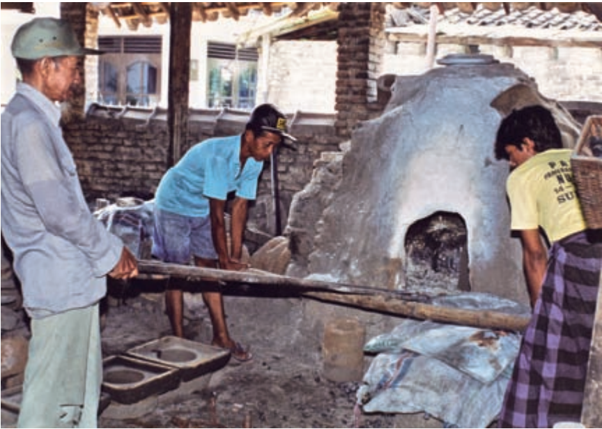
An old ceramic furnace used for brass casting in Batur village. (below) An old Chinese box bellows in Batur village; it is built into the right side of the kiln.
