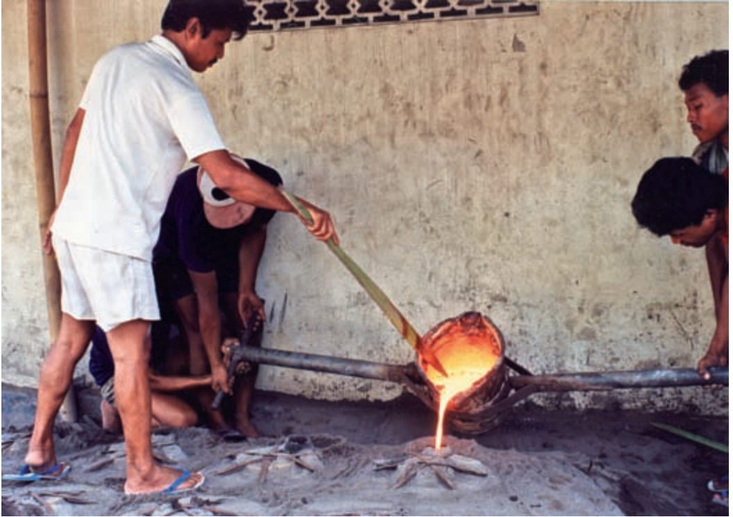
Pouring molten iron into earth molds, Batur village.
