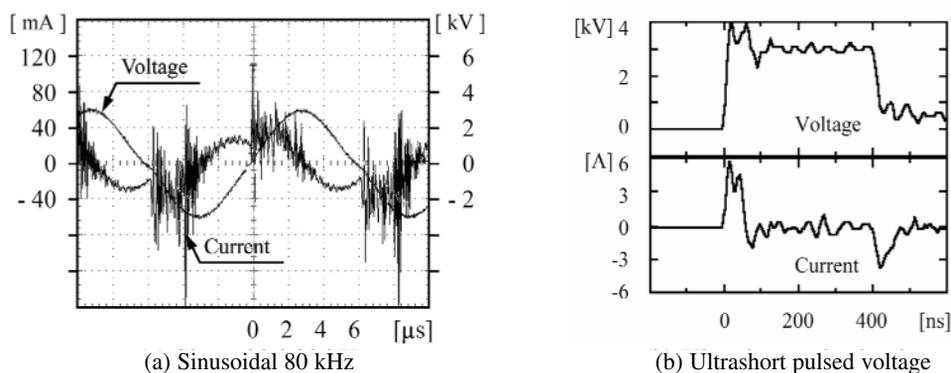
Fig. 1 Voltage and current waveforms.
