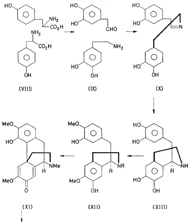
constructed from two different moieties. 1-Labelled 3,4-dihydroxy-2-phenylethylamine gives morphine labelled only at position 16<sup>15</sup>. The results are best explained if the morphine molecule is constructed from one molecule of the phenylamine and one molecule of 3,4-dihydroxyphenylacetaldehyde (see IX) giving the Schiff's base (X). By rearrangement the latter would afford norlaudanosoline (XIII) which has been proven to be an efficient precursor of morphine<sup>16</sup>.
