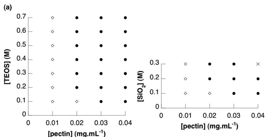
**Fig. 1** Phase diagrams of pectin with (a) TEOS and (b) silicates after 24 h: no gel formation (diamonds), gel formation (dark dots), inhomogeneous gels, or precipitates (crosses).
