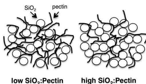
**Scheme 2** Proposed structure of silica–pectin hybrid materials at low and high SiO<sub>2</sub>:pectin ratio.
