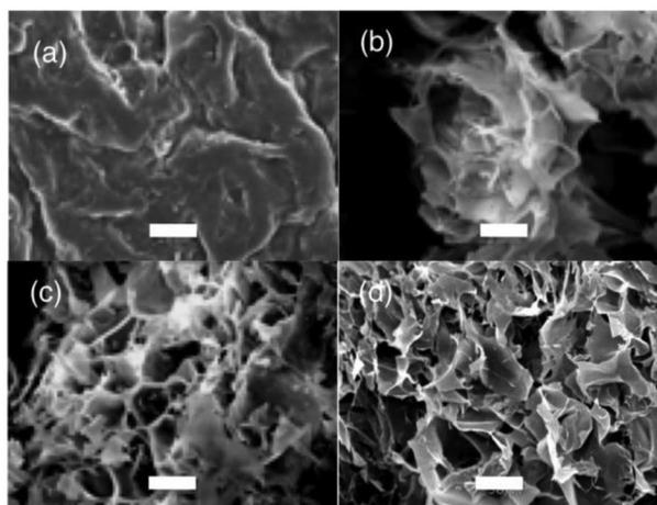
Fig. 4 SEM images of selected pectin–silica materials: (a) **P4T1**, (b) **P4T7**, (c) **P2T7**, (d) **P4Si** (scale bar = 20  $\mu\text{m}$ ).
