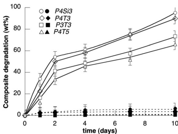
Fig. 6 Degradation of selected pectin–silica gels in acidic conditions (pH = 4) without (dark symbols) or with added enzyme (open symbols).
