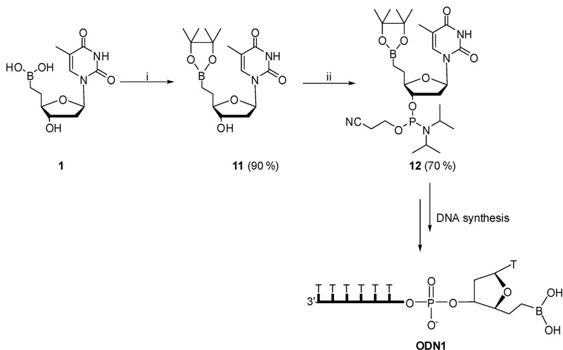
**Scheme 2** Synthesis of a borono-oligonucleotide. (i) Pinacol, THF; (ii) 2-cyanoethyl *N,N*-diisopropylchlorophosphoramidite, DIPEA,  $\text{CH}_2\text{Cl}_2$ .
