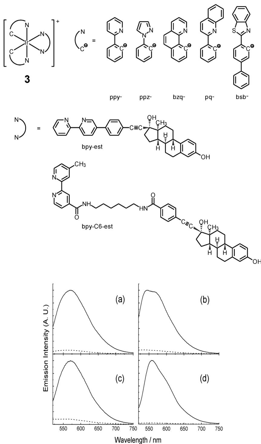
**Fig. 1** Emission spectra of  $[\text{Ir}(\text{N}^{\wedge}\text{C})(\text{bpy-est})]^+$  ( $\text{N}^{\wedge}\text{C} = \text{ppy}$  (a),  $\text{ppz}$  (b),  $\text{bzq}$  (c) and  $\text{pq}$  (d)) in the absence (dashed line) and presence (solid line) of  $\text{ER}\alpha$  (375 nM) in potassium phosphate buffer (50 mM, pH 7.4)/methanol (9:1) at 298 K containing  $100 \mu\text{M} [\text{Fe}(\text{CN})_6]^{3-}$ . Reproduced from ref. [18], with permission of the Wiley-VCH.
