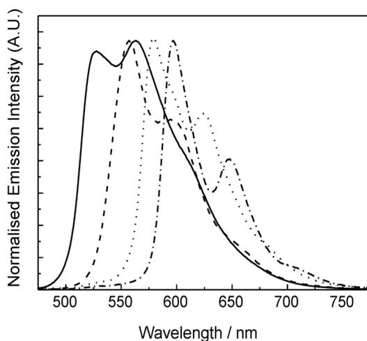
**Fig. 2** Emission spectra of  $[\text{Ir}(\text{N}^{\text{C}})_2(\text{bpy-CO-NH-C6-NH-biotin})]^+$  ( $\text{N}^{\text{C}} = \text{bt}$  (solid line),  $\text{bsb}$  (dashed line),  $\text{bth}$  (dotted line) and  $\text{bsn}$  (dash-dotted line)) in degassed  $\text{CH}_2\text{Cl}_2$  at 298 K. Reproduced from ref. [27], with permission of the American Chemical Society.
