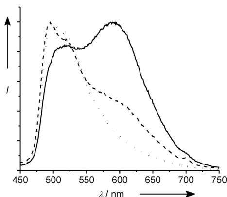
**Fig. 3** Normalized emission spectra of  $[\text{Ir}(\text{ppy-CH}_2\text{-NH-C}_4\text{H}_9)_2(\text{bpy-CONH-C}_2\text{H}_5)]^+$  in degassed  $\text{CH}_2\text{Cl}_2$  (solid line),  $\text{CH}_3\text{CN}$  (dashed line) and phosphate buffer (dotted line) at 298 K. Reproduced from ref. [32], with permission of the Wiley-VCH.
