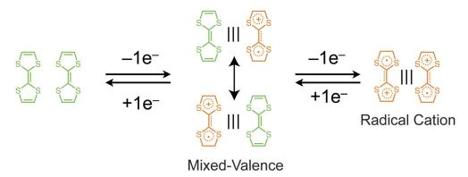
Fig. 3 The stepwise oxidation of adjacent TTF units results in the formation of firstly a mixed-valence dimeric state in which the radical character is shared equally between both units. The second oxidation results in the formation of radical cation  $\pi$ -dimer in which overlapping SOMOs allows radical spin-pairing in this diamagnetic complex.
